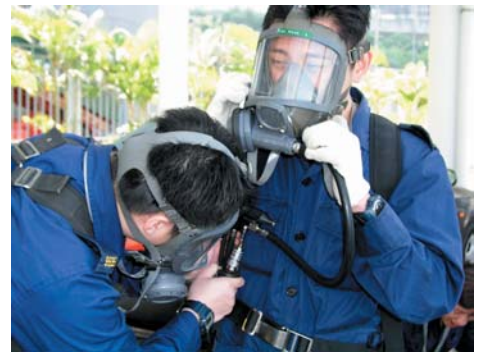
A trainee practising to use "Quick Coupling Connector" of his facemask to provide air to another breathing apparatus user.
