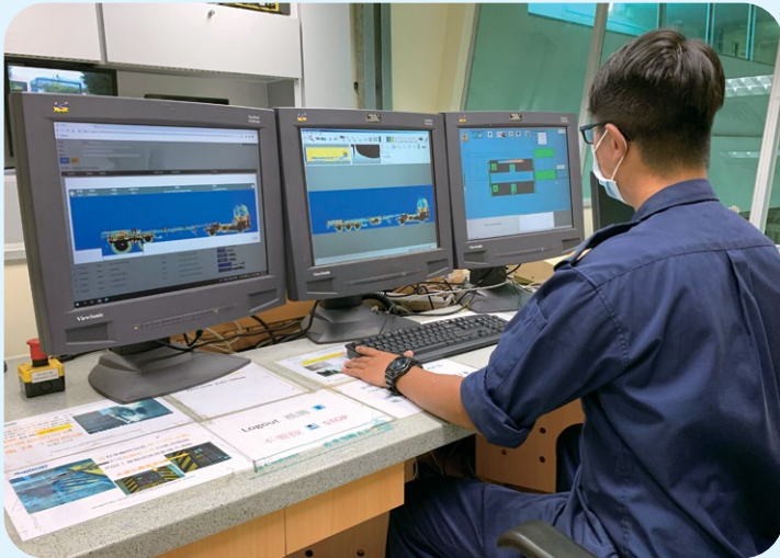
By using the powerful X-ray image comparison function of PRIME, X-ray image interpreter can make reference to the previous X-ray image of the same/similar cross boundary vehicle for instant image comparison.
