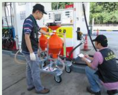
Customs officer checking the accuracy of a diesel dispenser by pumping out a pre-determined volume of fuel into a fuel-testing container.
