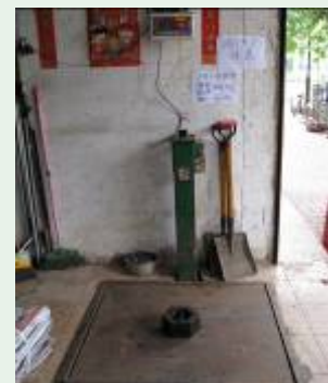
A defective electronic platform balance showing a reading of "9 kg" when checked with a standard mass of 10 kg.
