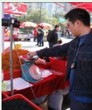
Customs officer checking the accuracy of a spring balance with a standard calibrated mass.
