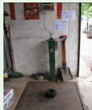
A defective electronic platform scale showing a reading of "9 kg" when checked with a standard mass of 10 kg.
