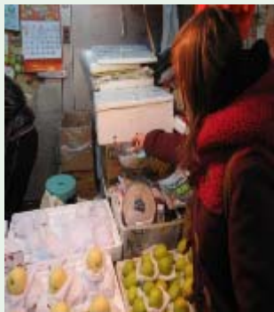
Customs officer checked the accuracy of a spring scale with a standard calibrated mass.
