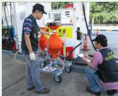
Customs officer checked the accuracy of a diesel dispenser by pumping out a pre-determined volume of fuel into a fuel-testing container.
