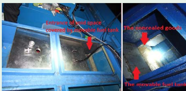
Movable fuel tank was used to cover the concealment on a speedboat.
