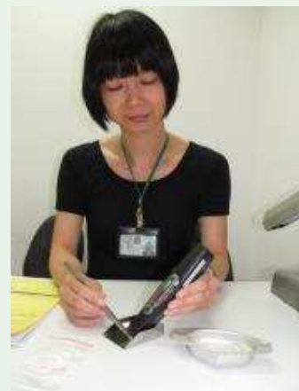
Officer conducting testing on rough diamonds with a diamond tester
