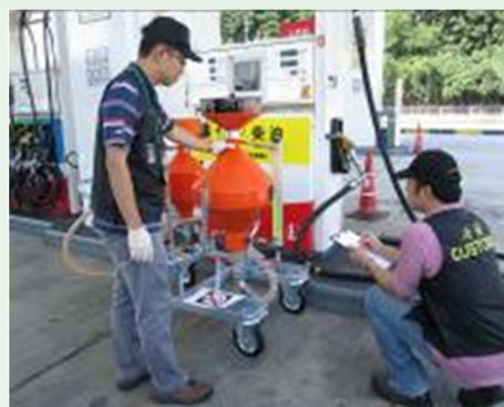
Customs officers checking the accuracy of a diesel dispenser by pumping out a pre-determined volume of fuel into a fuel-testing container
