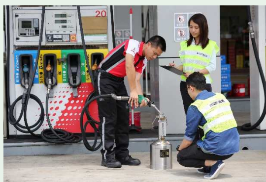
Customs officers checking the accuracy of a diesel dispenser by pumping out a pre-determined volume of fuel into a fuel-testing container
