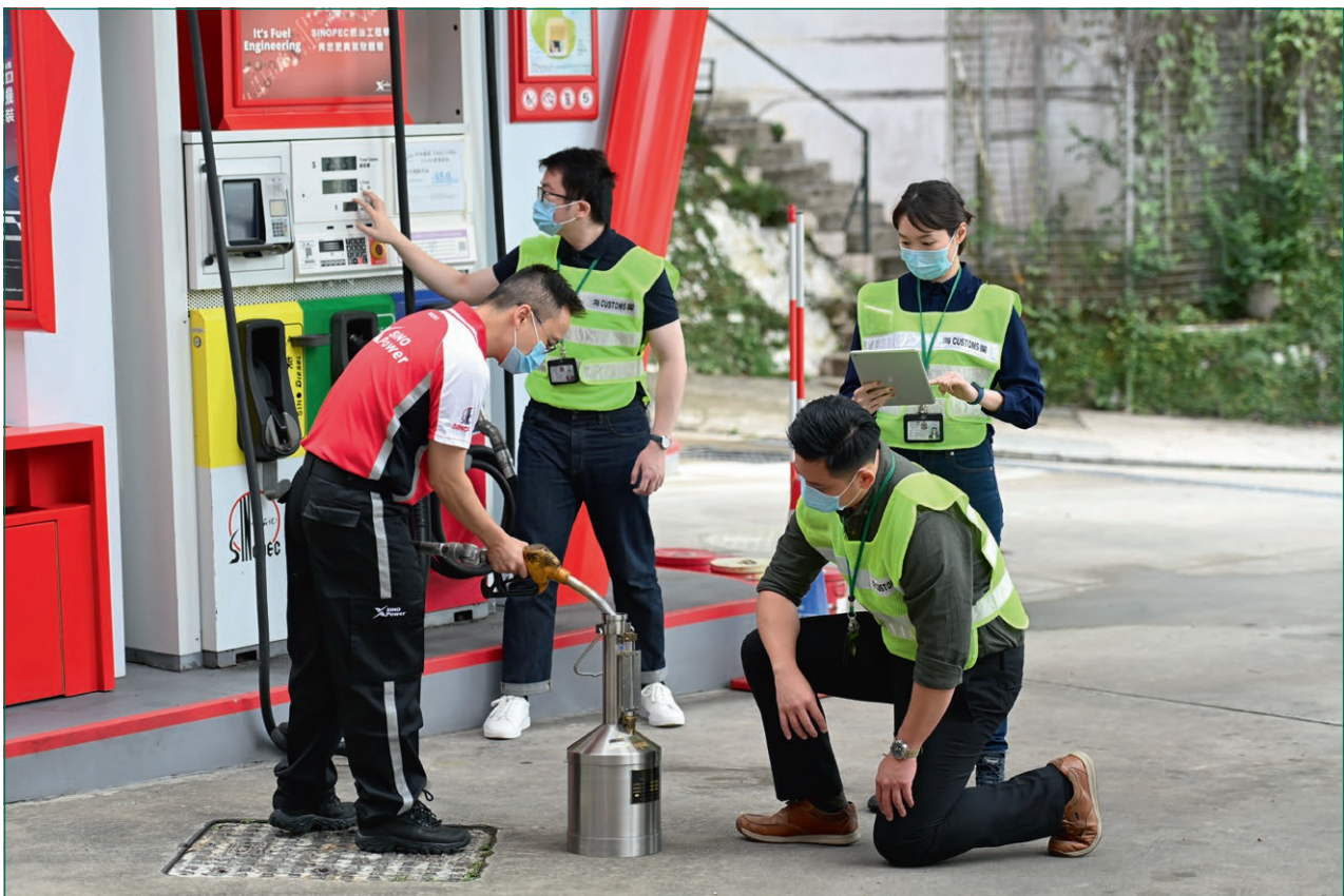
Customs officers checked the accuracy of a diesel dispenser by pumping out a predetermined volume of fuel into a fuel-testing container.
