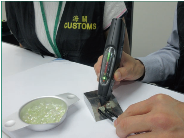
Customs officer used a tester to authenticate the genuineness of rough diamonds.
