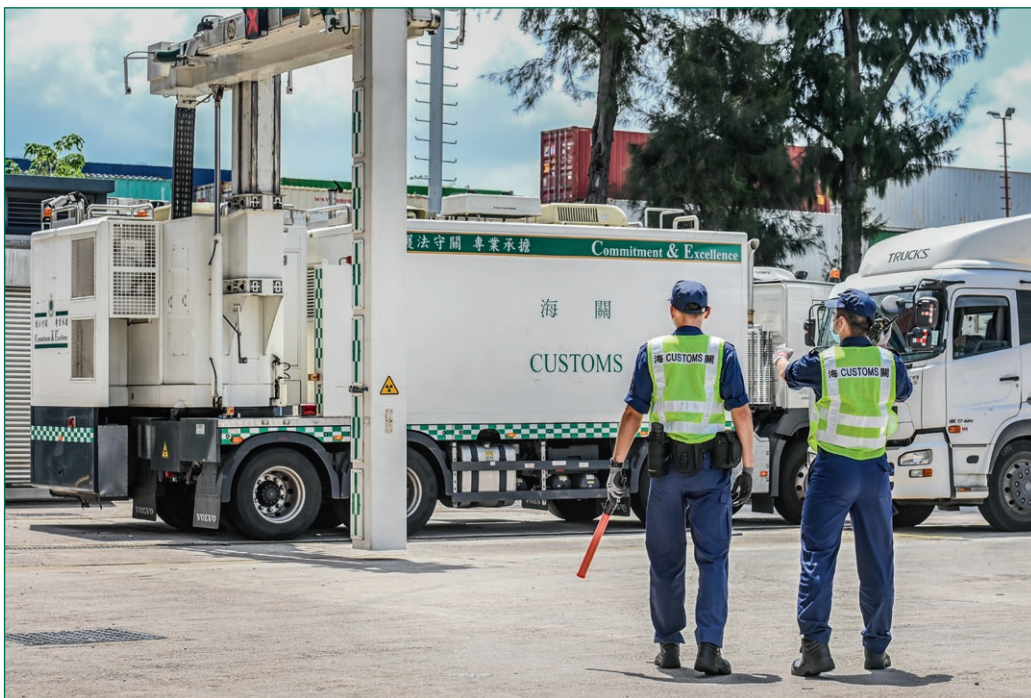
Customs officers used the Mobile X-ray Vehicle Scanning System to perform X-ray scanning of containerized cargo at the Kwai Chung Customhouse.
