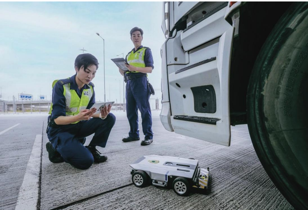
Customs officers utilised a “Smart Under Vehicle Robot” equipped with artificial intelligence for high-definition image comparisons to detect contraband concealed beneath the vehicle.
