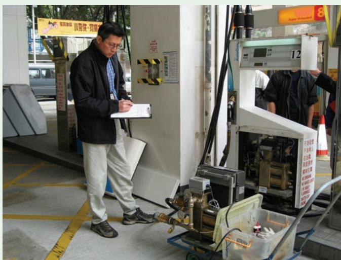
Customs staff member verified the accuracy of a Liquefied Petroleum Gas dispenser at a gas refilling station.
