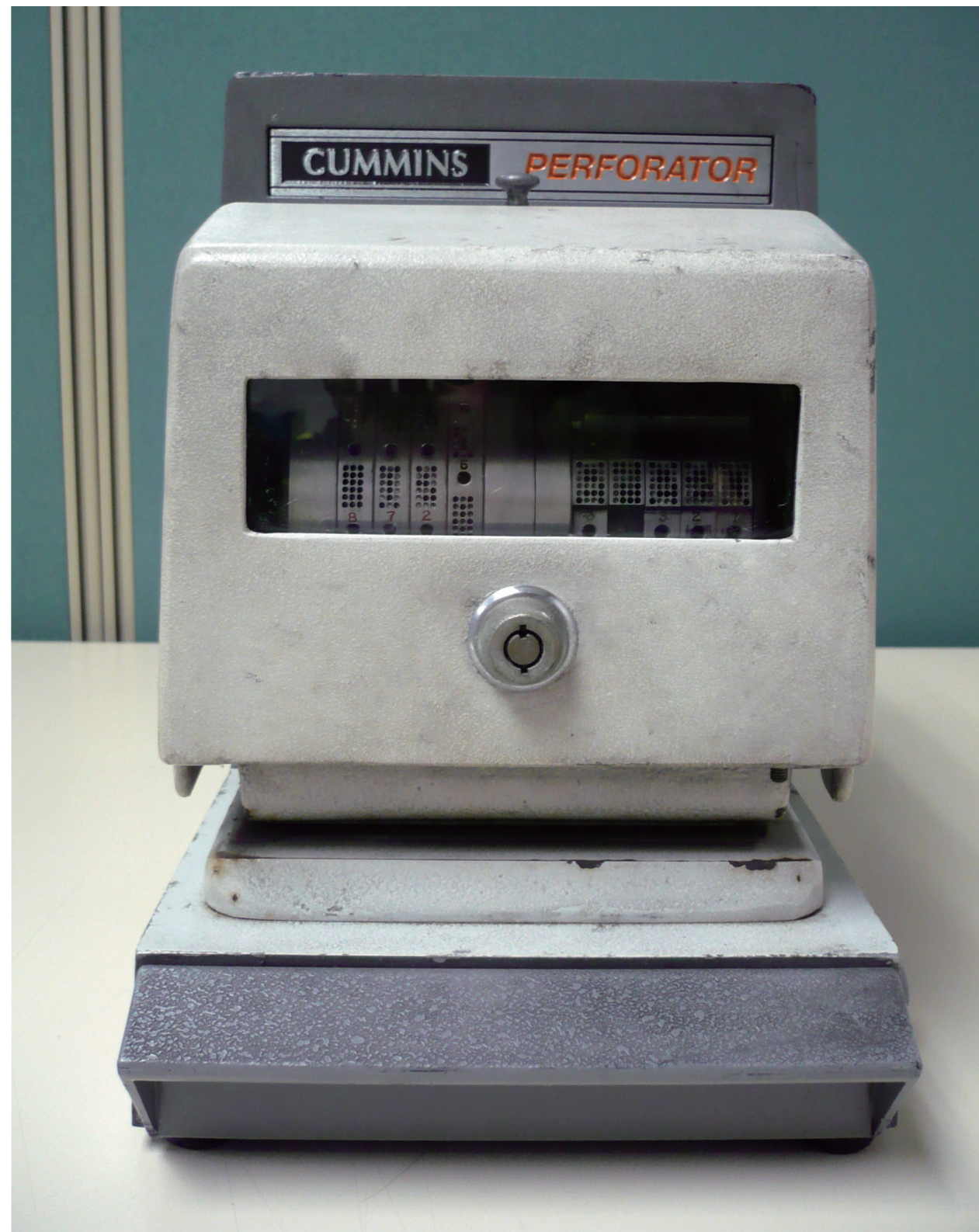
【圖七】 穿孔機曾在陸路口岸使用，為每套出入口載貨艙單打孔，編印獨一無二的載貨艙單編號，減省以往由人手蓋印的工序。 [Picture 7] Perforator was used at land border control points to perforate at one time the whole set of import and export cargo manifests with a unique number, which saved the procedure of chopping each cargo manifest by hand
