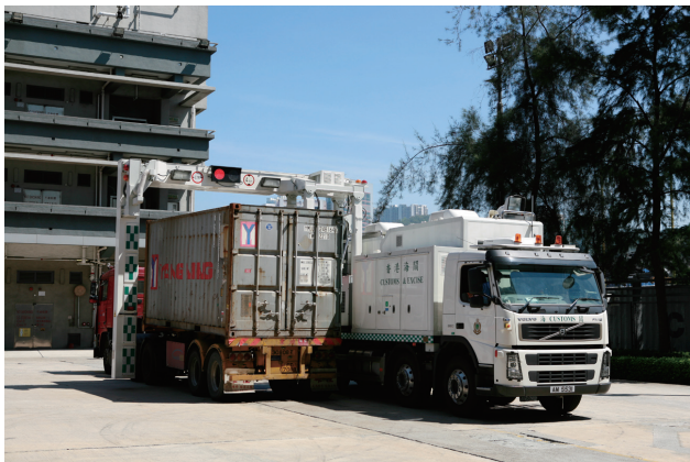
【圖六十一】 流動 X 光車輛掃描系統正在掃描一輛貨櫃車 [Picture 61] The Mobile X-ray Vehicle Scanning System scans a container truck with its X-ray detector arm
